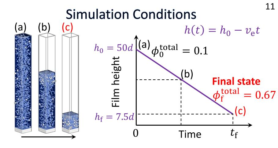
• Particle drying Péclet number (L) Pe =  $\frac{(\text{Drying rate})}{(\text{Diffusion rate})} = \frac{v_e}{D/d} = \frac{v_e d}{D}$ Simulation: Pe =  $0.3 \sim 1000$
