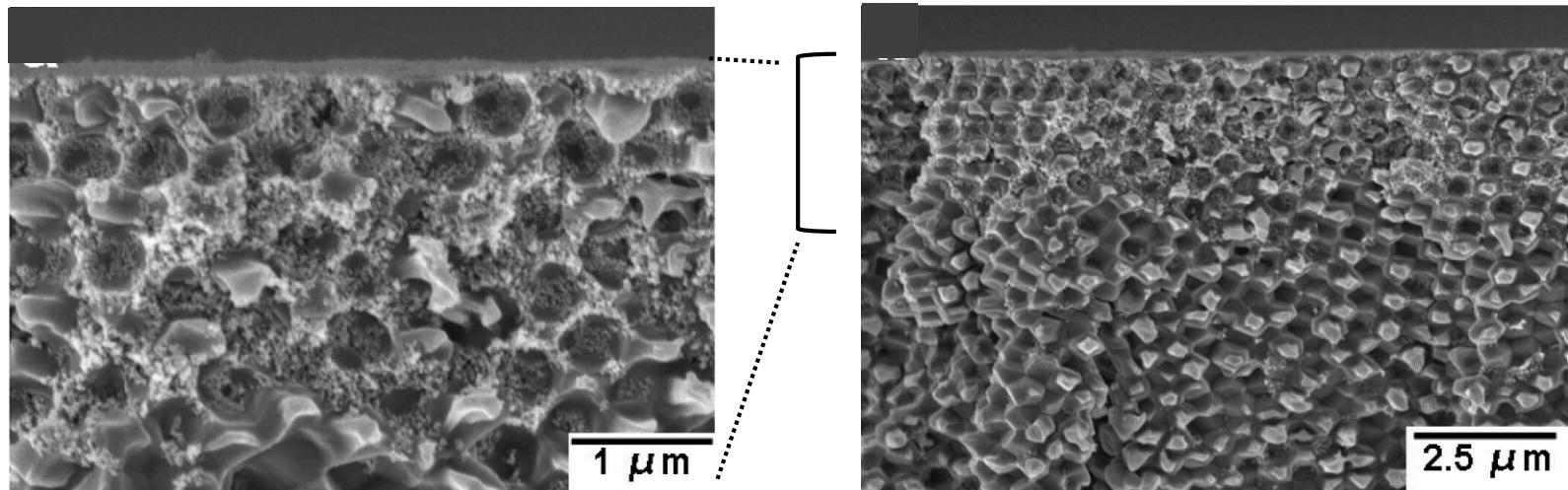
SEM images of the cross section of a dried silica (20 nm) / latex (550 nm) coating
