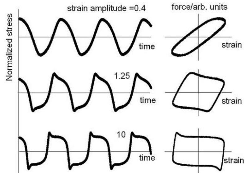
**LAOS** (Large Amplitude Oscillatory Shear;  $\gamma_0 \gtrsim 1$ )
