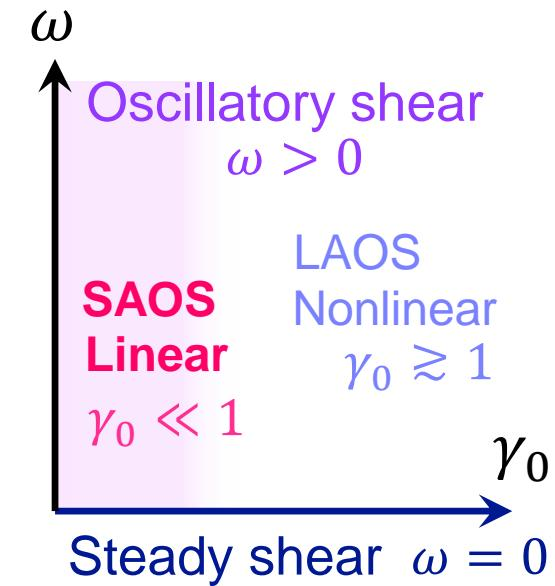
**SAOS (Small Amplitude Oscillatory Shear;  $\gamma_0 \ll 1$ ) → Linear response**
